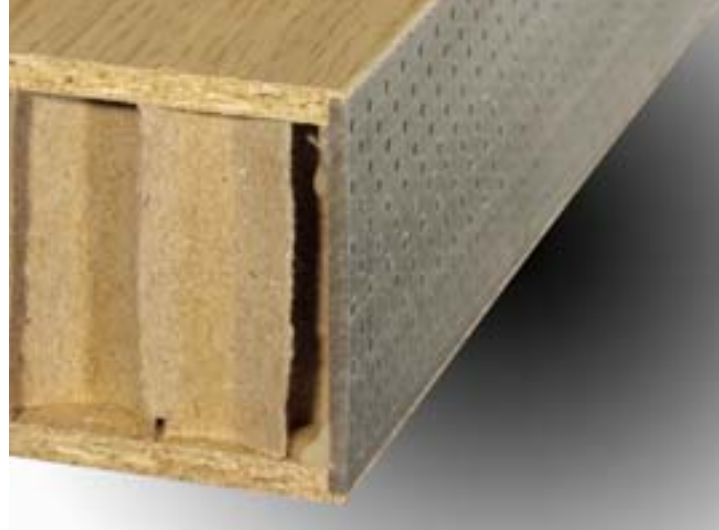
Lightweight boards with 4 mm decks: This is where the Doellken Bonding Edge comes into play. The supporting edge is inserted in grooves that are pre-milled.
